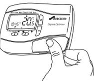
**How to fit the batteries**
