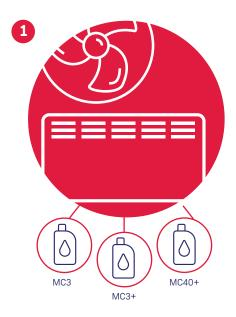
A flush should be completed on new systems and when repairing existing ones. Magnetite capture and radiator agitation can improve speed and effectiveness.
